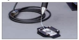
In-line solution heaters are the most direct way to warm solutions flowing into a series of devices. Small size allows placement close to imaging and recording chamber so as to minimize convective heat losses.
