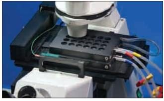
The Electric CO<sub>2</sub> Microscope Stage Incubator fits all the XY stages on the market, and it is suitable at the same time for high magnification microscopy and multipoint experiments. A wide choice of interchangeable inserts adds flexibility to the equipment and allows the use of any cell culture support (Petri-dishes, glass slides, mutiwell plates, etc.).
